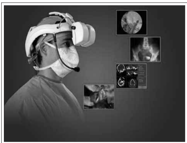
Figure 3. Three-dimensional head mounted surgical display into which images can be imported or presented in real time as imaged. (Courtesy of Viking Systems, Inc., La Jolla, CA).
